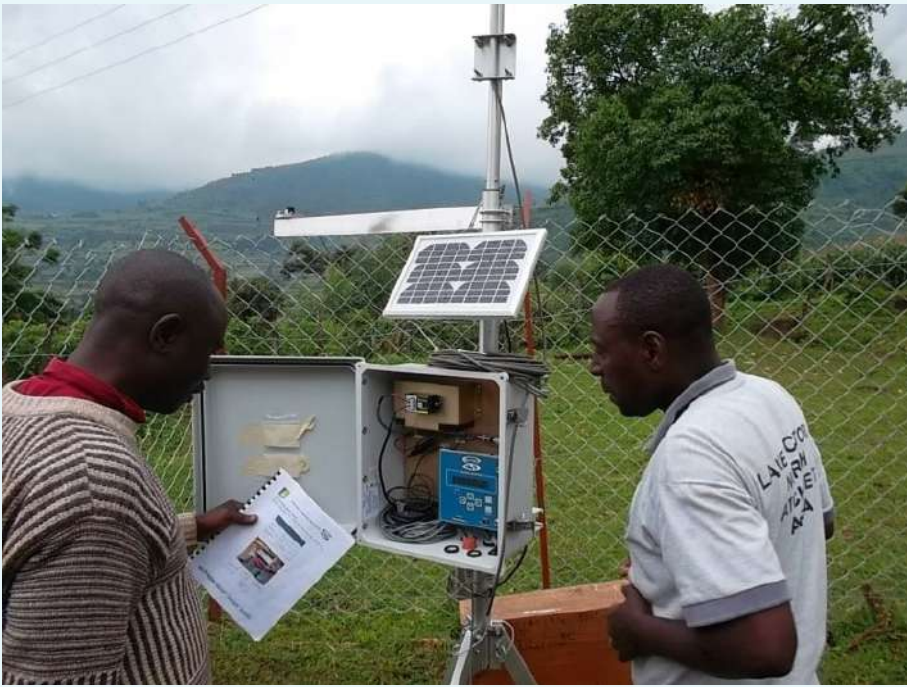
WRMA OFFICERS CONFIGURING AN AUTOMATIC WEATHER STATION
